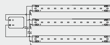
Parallel connection with return terminal block
