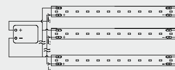
Parallel connection with return terminal block
