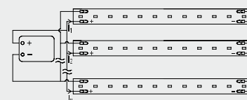
Parallel connection with return terminal block
