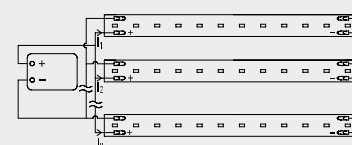
Parallel connection with return terminal block
